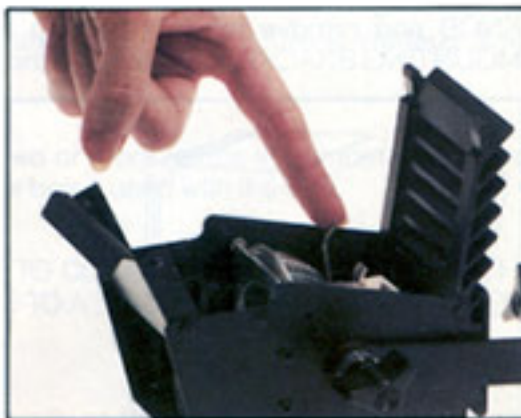
5. Push the LAMP EXTRACTOR LEVER to the rear of the housing. This will raise the lamp part way from the socket, allowing you to grip the front rim of the reflector on the top side.
