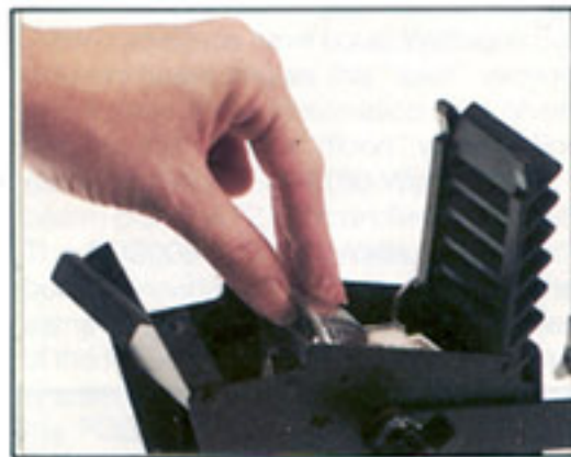
6. Grasp the top edge of the reflector and lift the lamp straight up and out of the housing.
